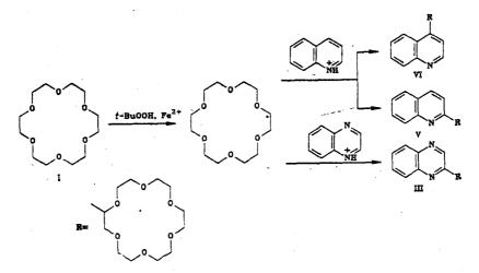
The extent of reaction of the aromatic base reaches 34-40%, with 80-85% reaction of the crown ether (I). The yield of (III) was 85% on base reacted.
